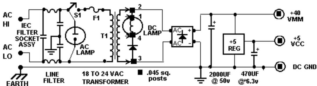
**NOTE: NEVER REPLACE FUSE! FUSE FAILURE INDICATES DRIVER FAILURE!**
