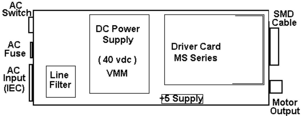
The SMD system is used with an external host computer or indexer card, or other device in positioning applications. The input connector supports controller input signals (Step & Direction) and a Limit-Loop safety.
