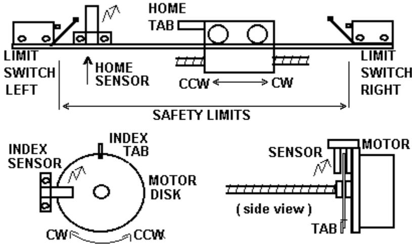
**ABORT LOOP FUNCTION.** In TMG systems, the ABORT loop is used to remove all winding power to the motor during an out-of-bounds condition. The ABORT feature can be used to provide hard-limits, emergency stop, door inter-locks, and other safety features. As the ABR input, to the driver, must be LO (ground) for the driver to step; opening the loop will stop (free) the motor regardless of the control logic. The diagram is typical of TMG "Fail-Safe, Hard-Soft" limit loops.
