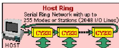
Host Ring and Party Line Networks are two of the various network connection schemes possible in this mode. These topologies will usually have a host computer controlling several CY233 nodes, with parallel device hardware connected to each node.
